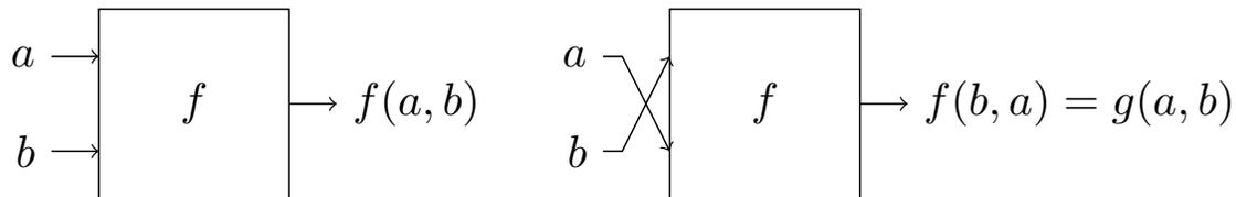
**Figure 14.25** A switching function of two variables
